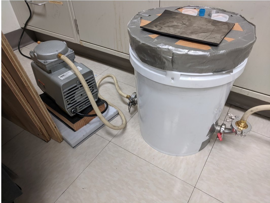
Figure A.2: Isolating transfer station from pump vibrations. Without any isolation, the vibrations of the diaphragm pump (shown on the left) would couple through the vacuum line to the transfer station, negatively impacting transfer quality. To mitigate this, the vacuum line is run through a 5 gallon bucket filled with sand (shown on the right).
